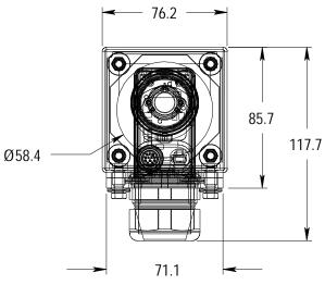
Material: Body-type 304 stainless Base-hard coat anodized 6061 Al Gaskets-EPDM
