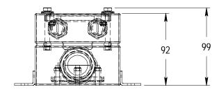
100% 316 stainless steel construction Glass or poly viewport window Designed for FDA food applications Drillable cord grip w/29mm dia opening 76mm height for camera/lens Air cooling/Air curtain options (kit)
