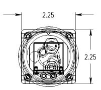
Rear plate includes Hirose bulkhead connector & 2 air fittings
