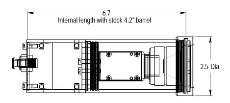
Rear plate can be changed to accomodate different cabling /cooling requirements
