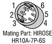
Figure 5: Hirose 6-pin Circular Male—Power Connector and Table 5: Hirose Pin Description
