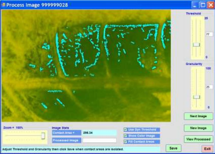
If the user checks the **Fill Contact Areas** option the software fills in the areas found in the operations instead of outlining the areas as is the default. This shows the actual contact area as calculated by the software. In some cases it may be easier to see the proper values of the Threshold and Granularity settings with this option either on or off.
