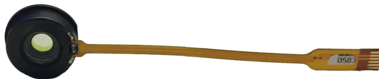
Figure 5: EL-3-10-XXX-26D-FPC with flex cable
