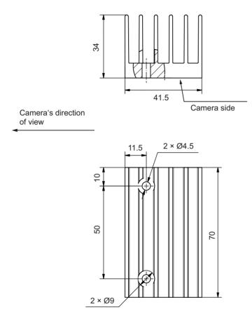
Fig. 1: Heat Sink for Basler boost Cameras Overview; Dimensions in mm
