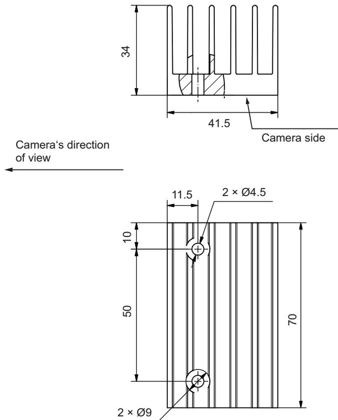
Fig. 1: Heat Sink for Basler boost Cameras Overview; Dimensions in mm
