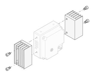
Fig. 2: Mounting Two Heat Sinks on a Basler boost Camera - One Heat Sink on Each Camera Side
