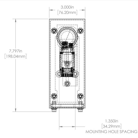
NOTE: MAXIMUM LENS DIAMETER 50MM MAXIMUM LENS LENGTH 58.5MM
