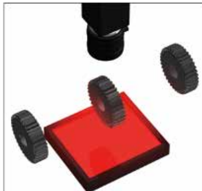
Gear processing inspection
