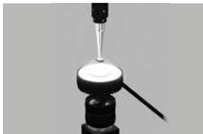
Alignment of electronic components on suction nozzle tips
