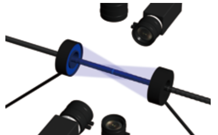
Visual inspection of medical endoscope tubes
