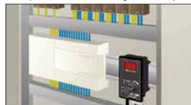
Example of DIN rail mounting in control panel
