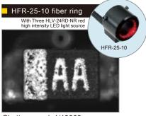
Shutter speed: 1/10000 Light Working Distance: 10 mm Light intensity: 70%
