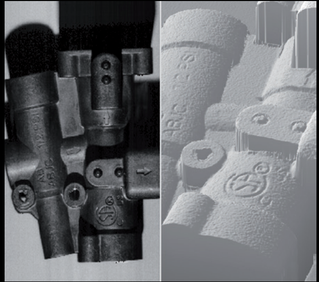
⚡ Resulting intensity image and 3D range map
