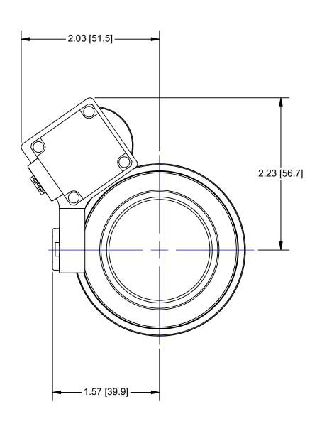
WORKING DISTANCE = 90mm FINE FOCUS TRAVEL = 10mm (OL SHOWN IN EXTENDED POSITION)
