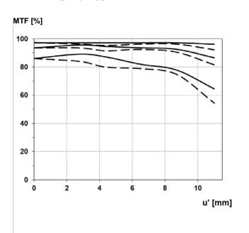
The Modulation Transfer (MTF) as a function of image height (u) and slit orientation (sagittal, tangential) has been measured with white light at spatial frequencies of R = 10, 20 and 40 cycles/mm.
