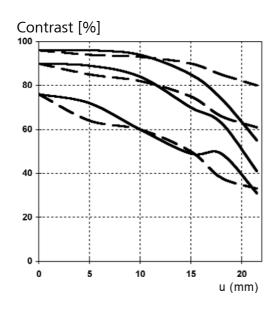
The Modulation Transfer (MTF) as a function of image height (u) and slit orientation (sagittal, tangential) has been measured with white light at spatial frequencies of R=10, 20 and 40 cycles/mm.
