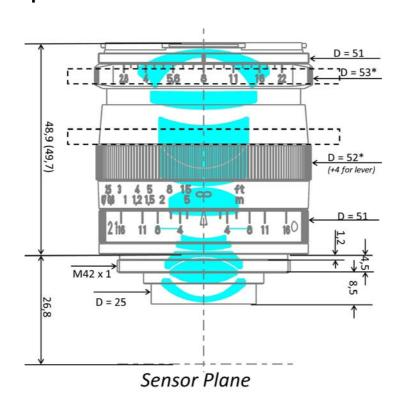
All values are valid for infinity. Values in brackets are valid for MOD. \*Excluding fixing screws. Length of fixing screws: 8 mm
