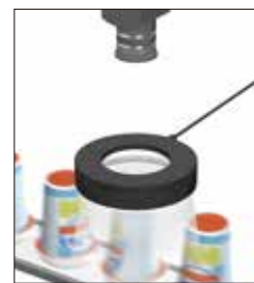
Condition of container bottom and text can be read.
