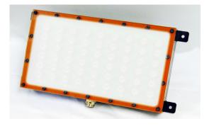
The MT-FL300x150 is a cost effective and "integrator ready" high power illuminator with versions that include a built-in constant current driver version (simply provide 24VDC to operate), Strobe-only version (simply provide 24VDC and trigger signal) and ULC-2 version (external constant current controller version for DC & strobe operation).
