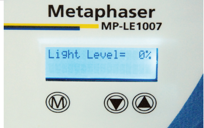
This image displays menu to change the intensity of the Metaphaser using the up and down arrows. (0% - 100%)
