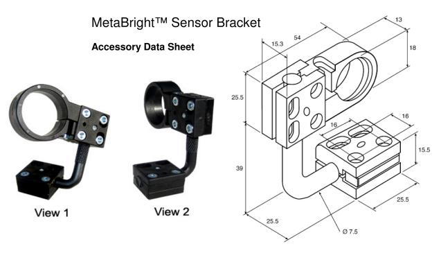
PART#: MBSB-30: For MBAFSL & LED Engine - 30mm Diameter Clamping Ring
