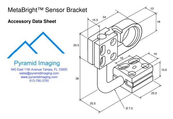
PART#: MBSB-30: For MBAFSL & LED Engine - 30mm Diameter Clamping Ring
