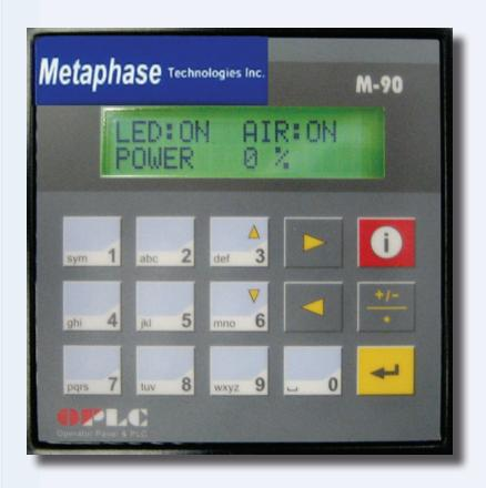
For manual intensity controller, light intensity settings are adjusted by tapping (or holding) either the 3 ▲ or 6 ▼ key.
