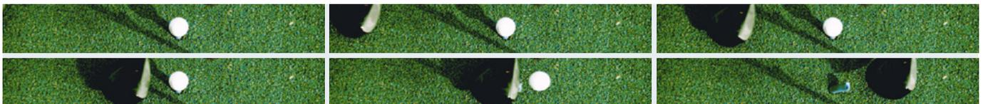
The detailed images show the golf club head at impact. This is the critical moment for the analysis, the moment of the impact. It determines the ball's takeoff velocity, direction of flight and spin. Here, the small image region meant the resolution could be reduced to 832 x 172 pixels. This allowed the MotionBLITZ EoSens® mini1 to reach a frame rate of 4,188 frames per second.
