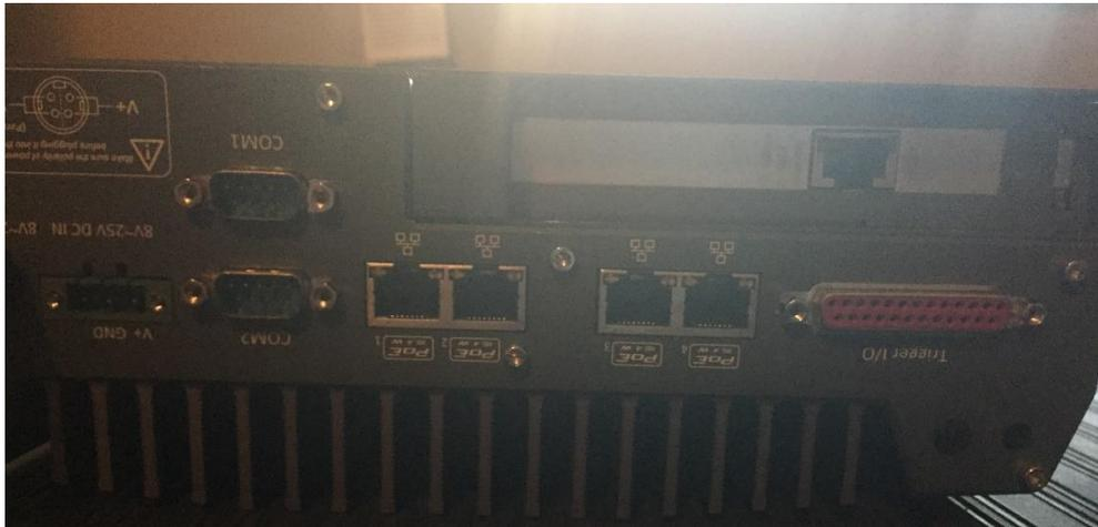
Figure 8: NIC installed in CPU housing.
