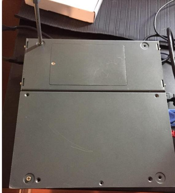
Figure 6: Disassembling CPU housing.
