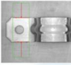
WebSpection® has the capability of measuring straight lines, circles, ranges, angles, etc. The software that controls WebSpection® provides contour tracking with high measuring accuracy and speed.
