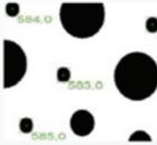
WebSpection® can count objects within only a few milliseconds. The only required command is the, so called, BLOB (Binary Large Object).
