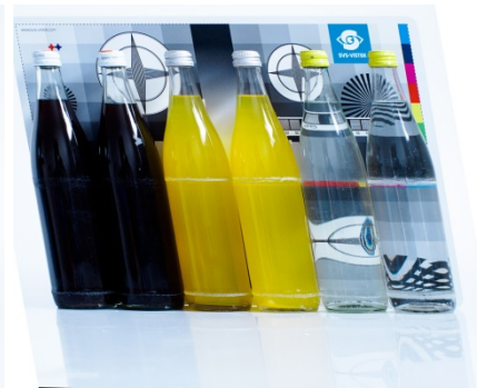
Figure 18 rolling shutter with moving objects (geometric distortion)
