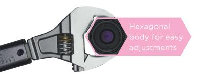
The hexagonal body of the lens makes it easy for anyone to correctly lock the lens into a camera with the use of a standard wrench or torque wrench. With a torque wrench it is possible to precisely tighten the lens to a camera with a specific amount of torque. It is then possible to replicate the same exact tightness in other vision systems using the VS-MCA lens series.
