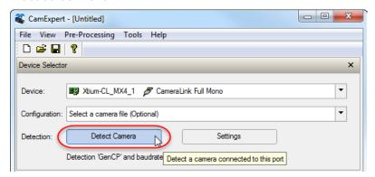
Both the frame grabber and camera parameters are displayed:
