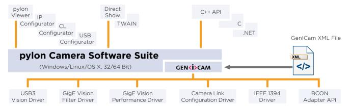
The architecture of the pylon Camera Software Suite is based on GenlCam Technology, which offers you easy access to the newest camera models and the latest features. Changes to an existing camera device in your application essentially become a plug-and-play process.
