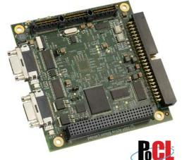
**Phoenix-D48CL** supports the Power over Camera Link (PoCL) functionality with *SafePower* and is able to provide power to PoCL enabled cameras via the Camera Link data cable thereby removing the need for a separate power supply. Conventional non-PoCL cameras are still supported.
