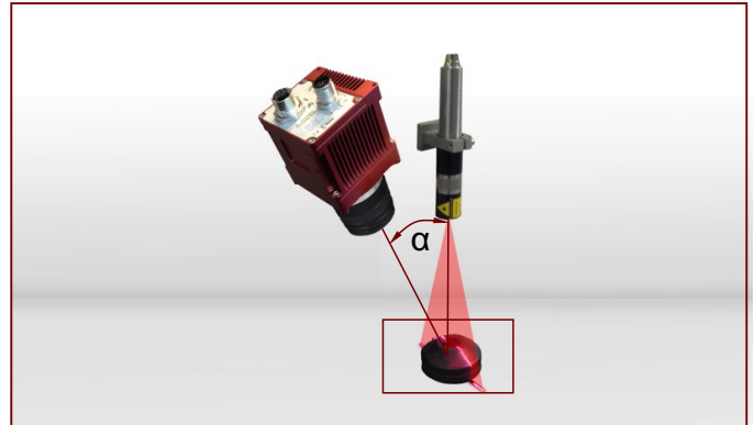
The C5 Sensor records the Shape of the Laser Line.
